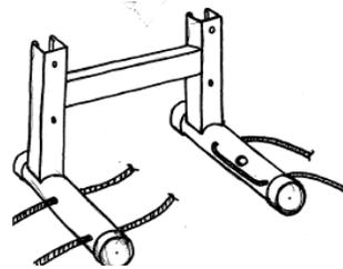
12. Insert the 1/2" –13 threaded rod through the hole in the bracket and thread on one of the 1/2" nuts.
