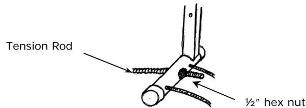
13. Place the tension bar on the other end of the 1/2" –13 threaded tension rod and thread the other 1/2" hex nut on.
