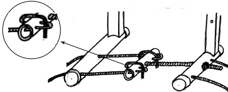
16. Tighten the ½" –13 nuts until the cables are tight and the bracket can no longer be moved on the tank.
