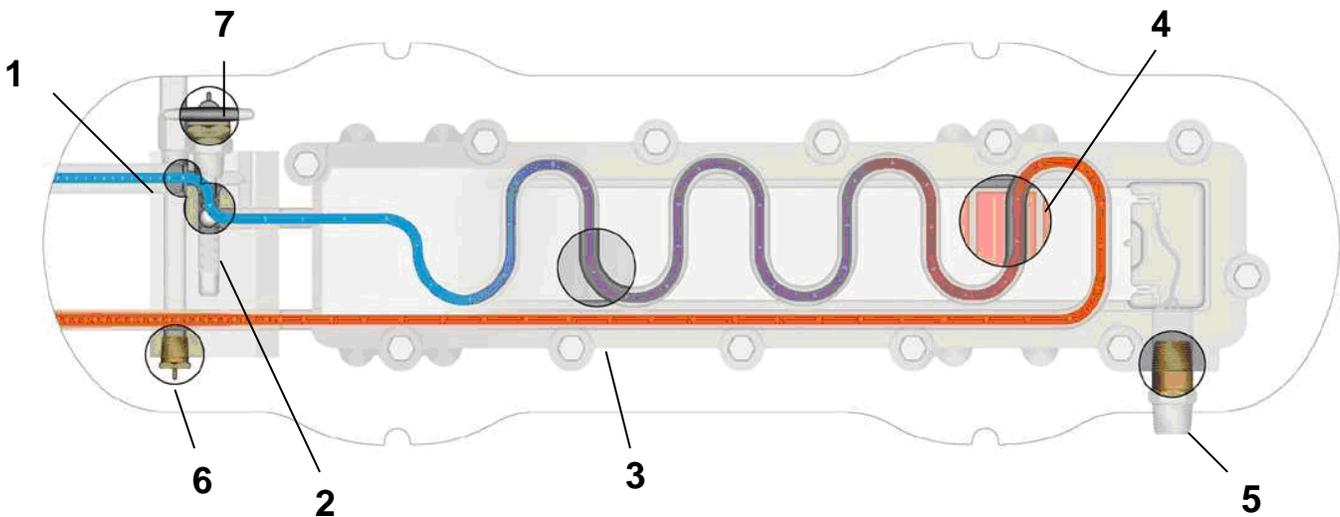
**Ref. 1** – Liquid LPG enters the inlet valve manifold where the inlet valve screen prevents debris from entering.
