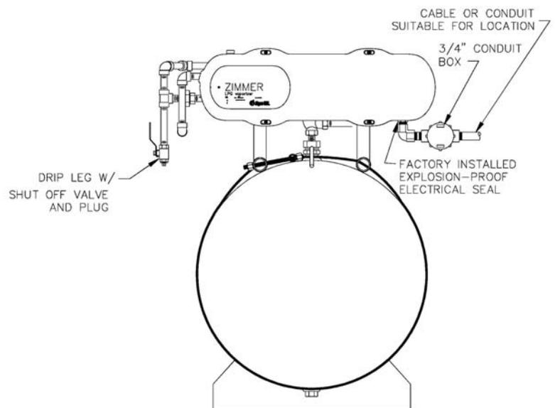
Typical Tank Mount Installation
