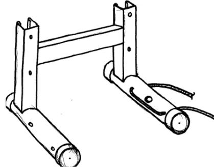
10. Place the *ZIMMER™* and bracket assembly onto the tank in the desired location.
