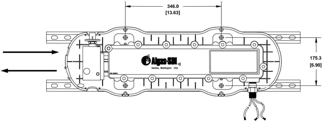
If mounted outdoors, the **ZIMMER™** must be mounted on a vertical or horizontal surface to maintain its enclosure rating. Use **Algas-SDI** Mounting Kit **P/N 80885**, or equivalent components, when mounting the **ZIMMER™** to a concrete, masonry or wood construction wall.
