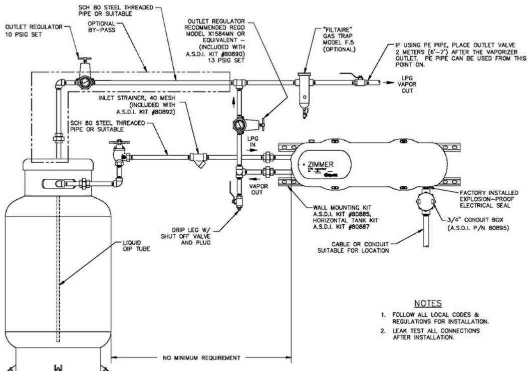
**Typical Installation with Stationary Cylinder**
