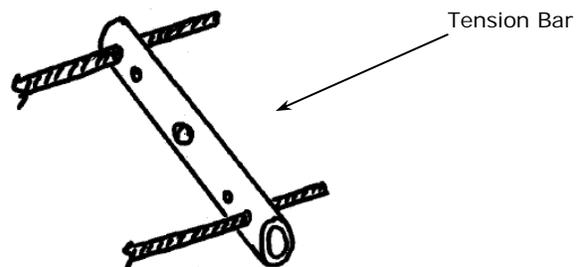
15. Feed the cable back through the inner holes. Save a small amount at the bend. Loop the cable back over the top of the tension rod and weave the cable through the small loop left at the bend. Pull the cable as tight as possible by hand.
