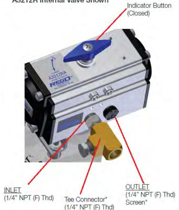
Position the actuator so that rain and other foreign matter can not enter the outlet.
